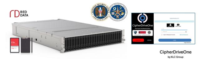
RedData's high-speed storage platform combines is a 2U Multi-Node Storage Server hardware platform that can hold up to 24 hot-pluggable CSfC listed Self-Encrypting Drives. It has 24 U.2 PCIe Gen 4 NVMe drive bays and is powered by an AMD EPYC Milan CPU. Each server module provides 8 DIMM slots and four x16 PCIe Gen 4 slots for flexible expansion.
